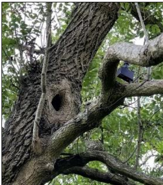
Figure 2: The articulating camera arm allows direct attachment to small limbs (if present, as shown in the left-hand picture) or to the buckle of a ratchet strap (as in the right-hand picture).
