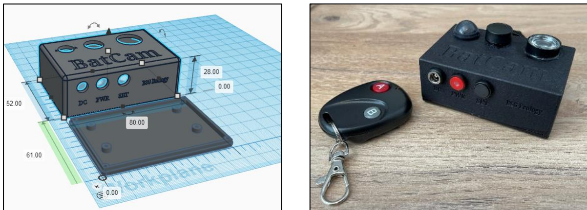
Figure 7: The screen grab on the left shows the case design in CAD software. The photograph on the right is the current BatCam with remote control fob.
