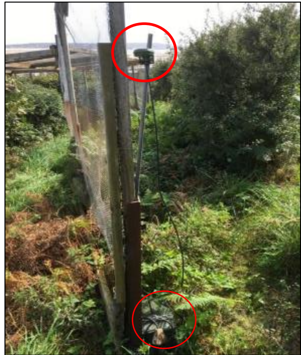
Figures 7 and 8: SM4 detector and microphone powered with 12v battery.
