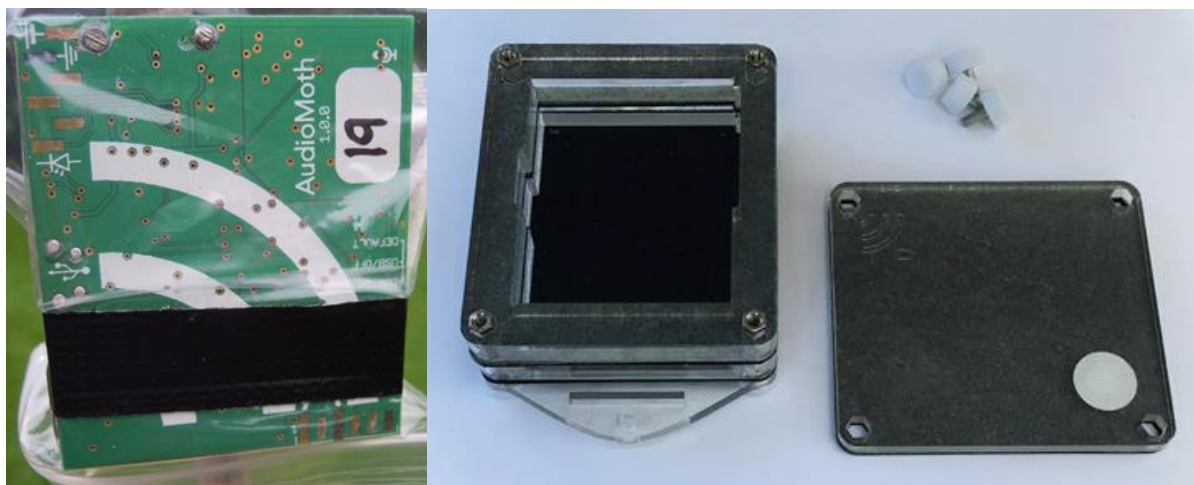
Figure 2. Options for weatherproofing AudioMoths, trialed by BCT prior to the current study. A push-close plastic bag ( left ) and an acrylic laser-cut case ( right ).
